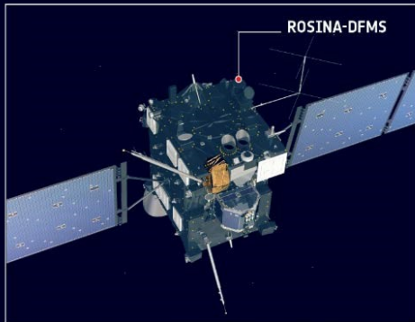
The measurements were made with the Rosetta Orbiter Spectrometer for Ion and Neutral Analysis Double-Focusing Mass Spectrometer (ROSINA-DFMS).
