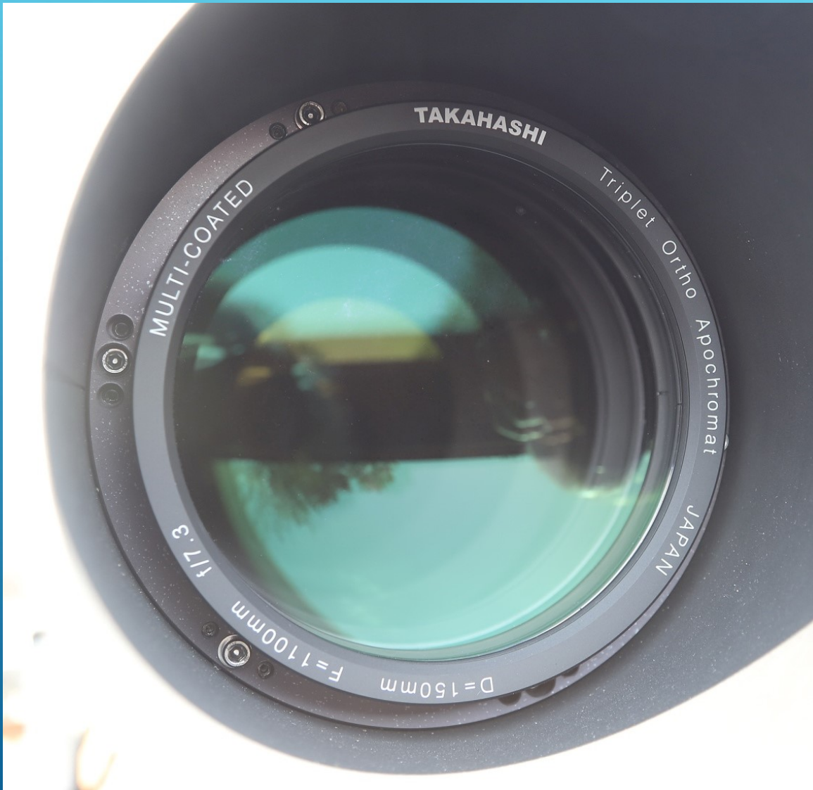
Takahashi TOA-150b, anno 2015. Triplet Ortho Apochromat, D=150mm, F=1100mm, f/7,3.
